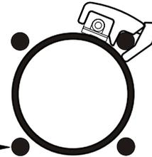
APPLY TO 32  $\phi$  TO 125  $\phi$  BORE TIE-ROD CYLINDER (TIE ROD SIZE FROM 5  $\phi$  TO 12  $\phi$  DIAMETER)
