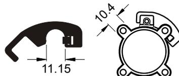
Apply to 32  $\phi$  to 40  $\phi$  ISO Profile Cylinder
