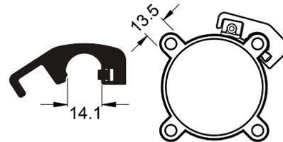
Apply to 50  $\phi$  to 63  $\phi$  ISO Profile Cylinder
