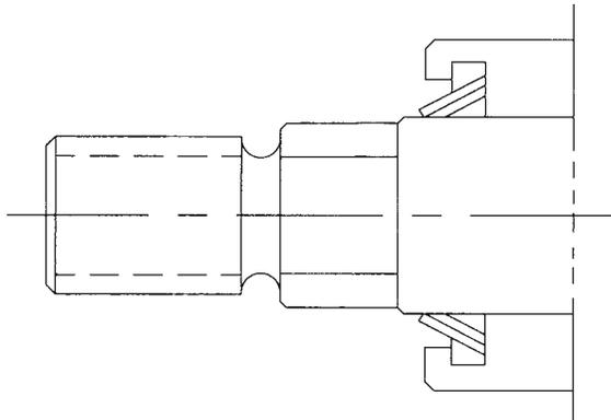
A rod scraper may be necessary when the cylinder must endure paint overspray, weld splatter or flyash.
