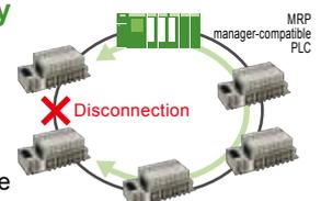
\* This device is compatible with MRP client function. When connecting in a ring, MRP manager function-compatible PLC is necessary.
